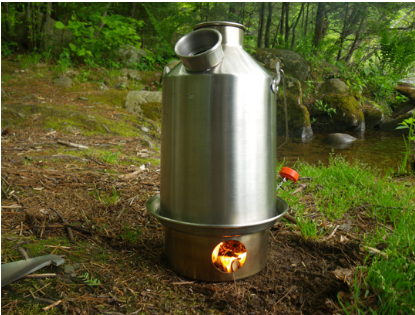
Above: A Kelly Kettle is used to boil water, which can be used to cook rice, pasta, etc. A similar design is called the Ghillie Kettle.
