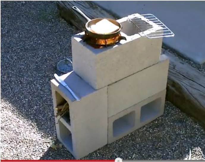
Above: Rocket stove made from cinder blocks
