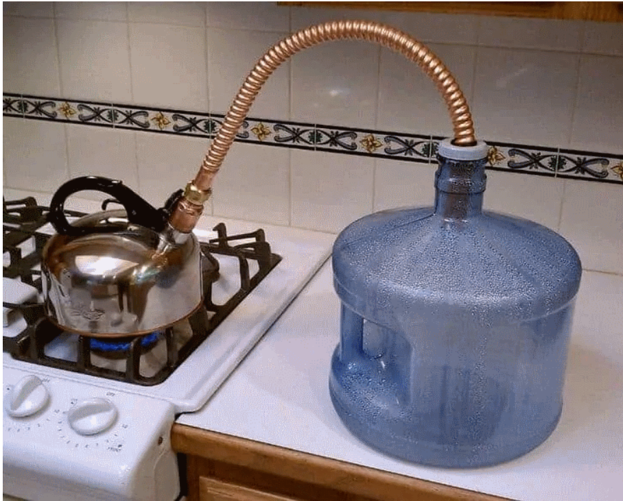
Above: One type of simple water still. The blue water jug really should be in a pan or bucket of cool water to enhance distillation.
