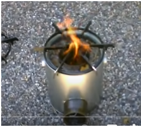
Above: Rocket stove made with gravel as a filler. See video below.
