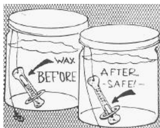
Above: Here's a device to tell you when water has reached a pasteurized temperature using the sun.
