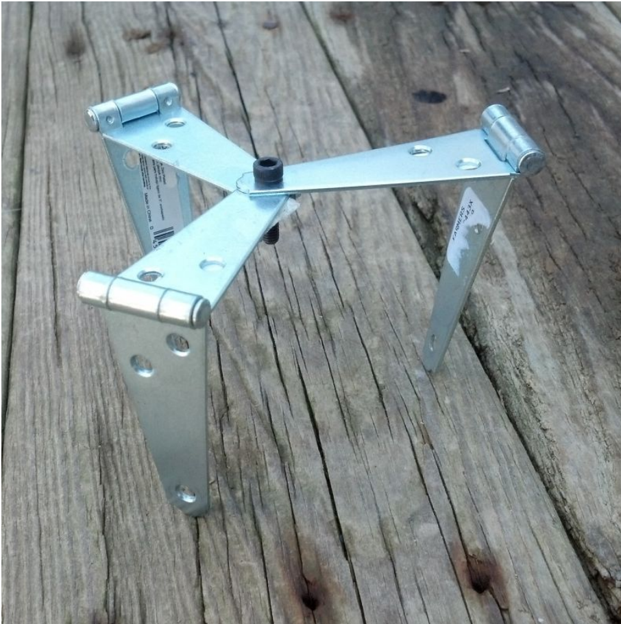
Above: Pot holder made from hinges. This style hinge only opens 3/4 of the way. This appears to be a "gate hinge".
