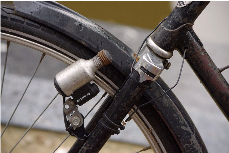
Above: Dynamo on a bicycle. This one does not appear to touch the tire so it may not generate power.
