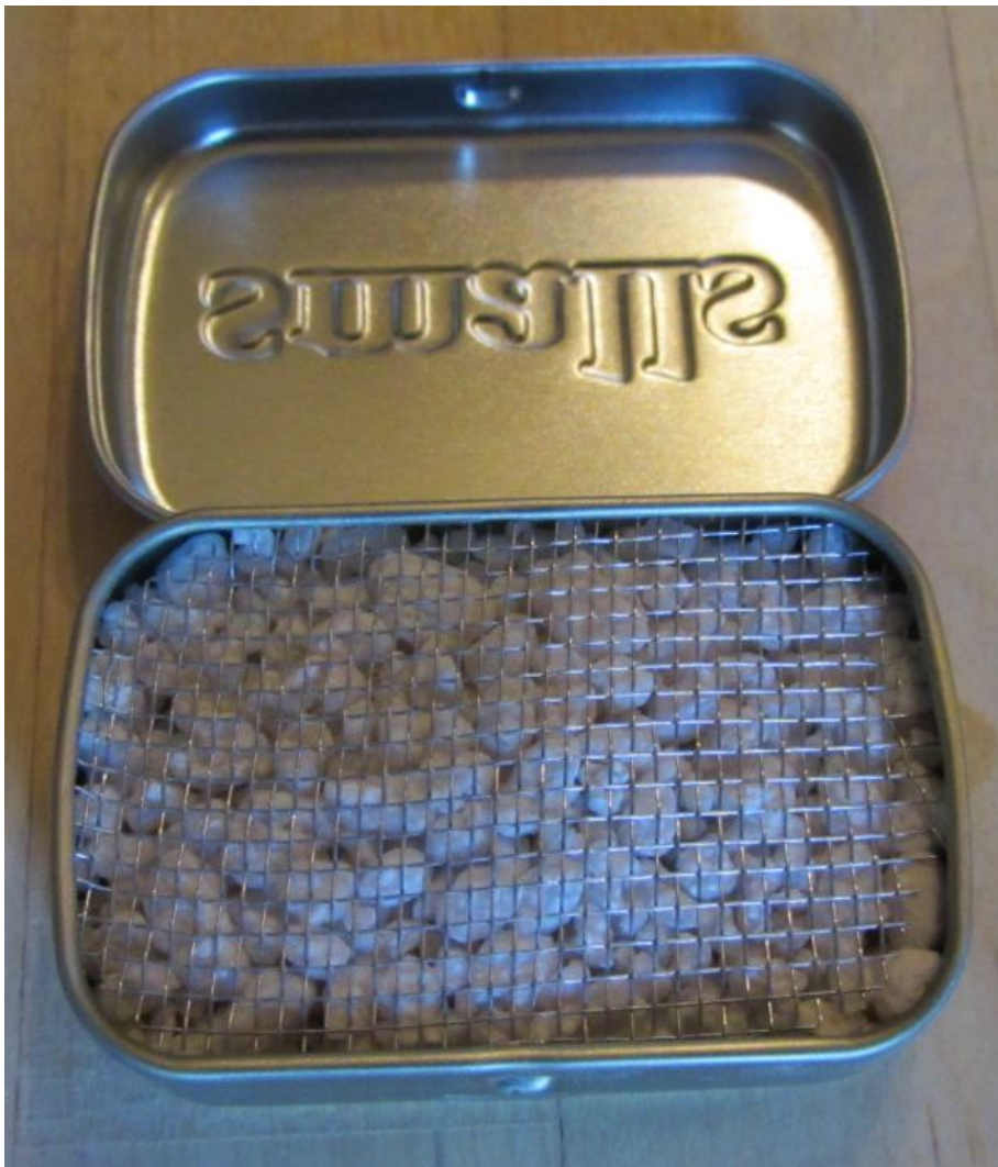
Above: Alcohol stove made from mint tin and rock wool. You will need a stand for this to raise the pot up about 2 inches, pots should not be placed directly on top of this stove because they will block air flow.
