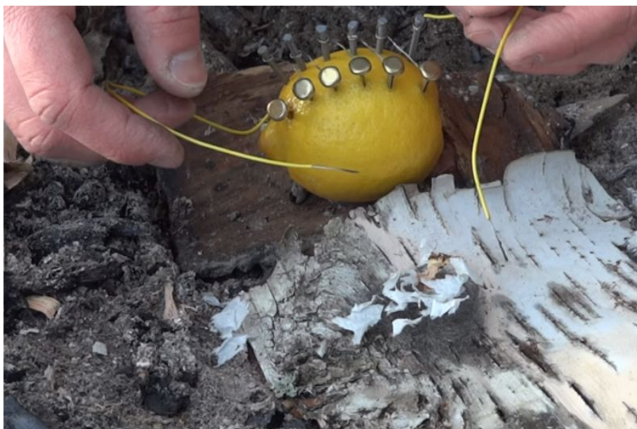
Above: Lemon battery trying to start a fire. A battery requires 2 different metals to work. The 2 different metals used in this image appear to be zinc nails and brass. "Galvanized" nails are coated in zinc.
