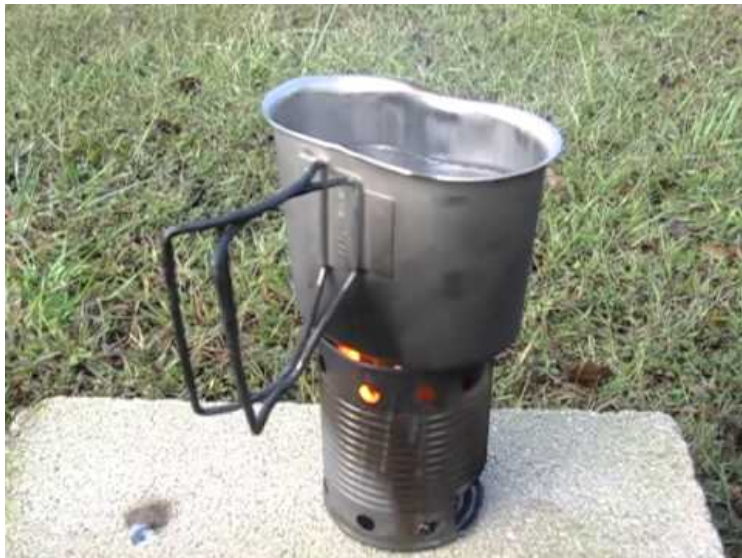
Above: Small hobo stove made from one can
